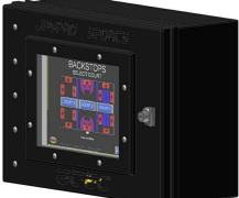
The ETEC offers state-of-the-art high resolution color LCD touchscreens, available in three sizes, 6", 8", or 10.4". The ETEC is mounted in an enclosure behind a polycarbonate window to provide protection to the screens. The enclosure may be recessed within the wall or surface-mounted to easily retrofit the system into existing facilities. Enclosure size is 16-1/4" W x 12-3/8" H x 7-5/8" D with a optional locking door.
