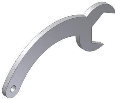
Figure 4-8: Spring tension adjustment wrench
